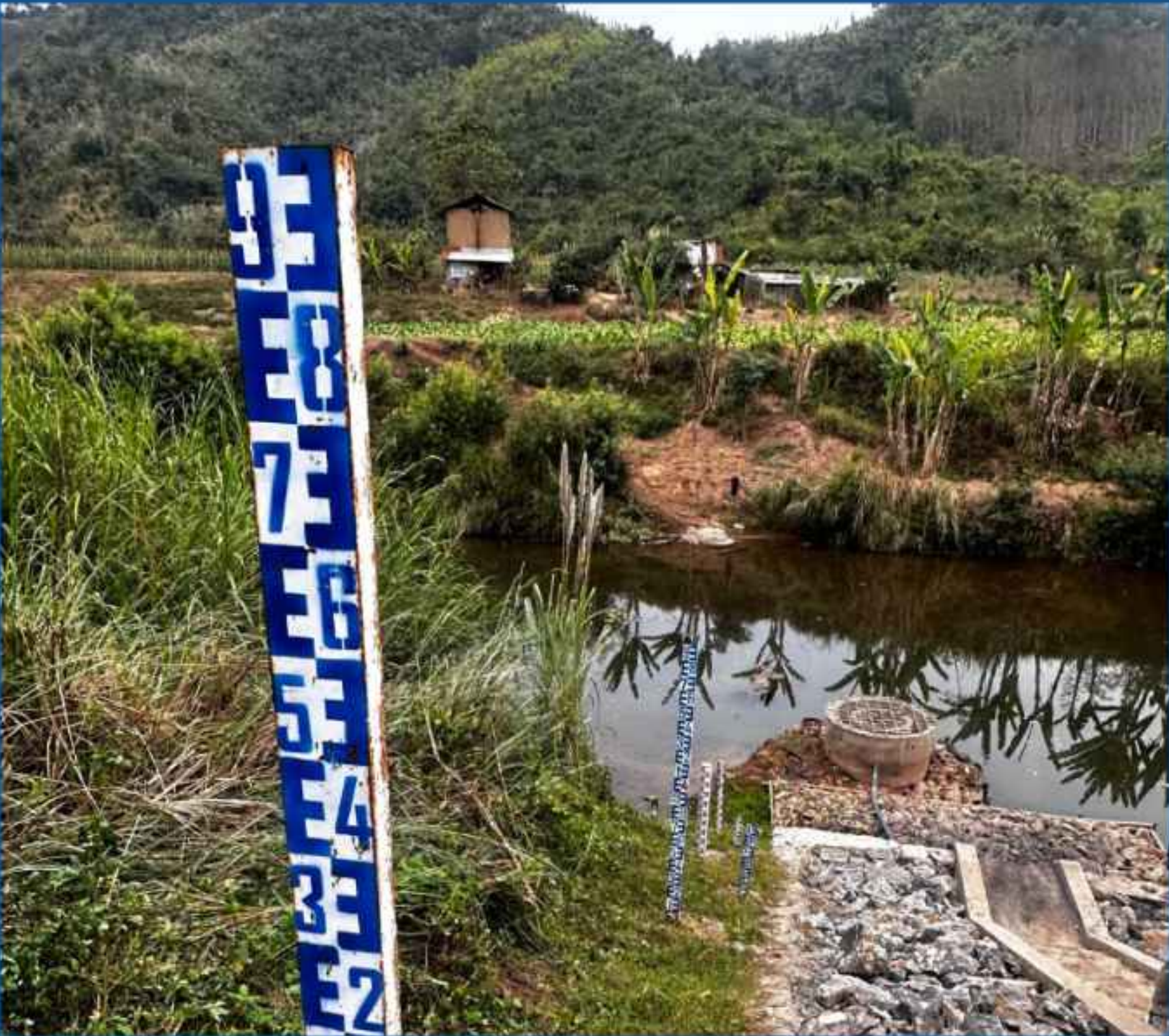
A river gauge installed on the Kor River in Xay District, Oudomxay Province, provides early warnings to the community through an automatic station, assisting the Hydrometeorological Office in delivering timely alerts (Credit: @sanjay pariyar/ UNDRR)
